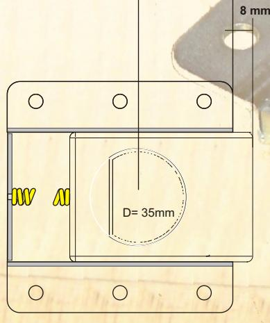
This versatile sliding latch can be used in a variety of functions such as service hatches, doors, lids, etc. Special care has been taken in the development of this product to keep it flat, thereby taking up as little space inside as possible.
